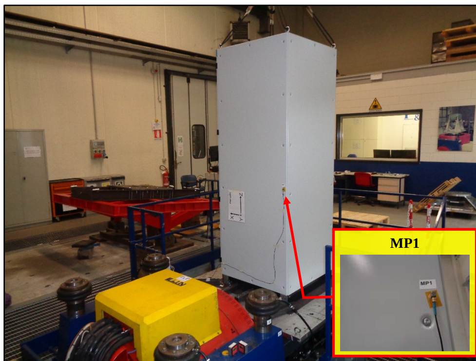
Photo 7 - Measuring points on the unit (MP1)
