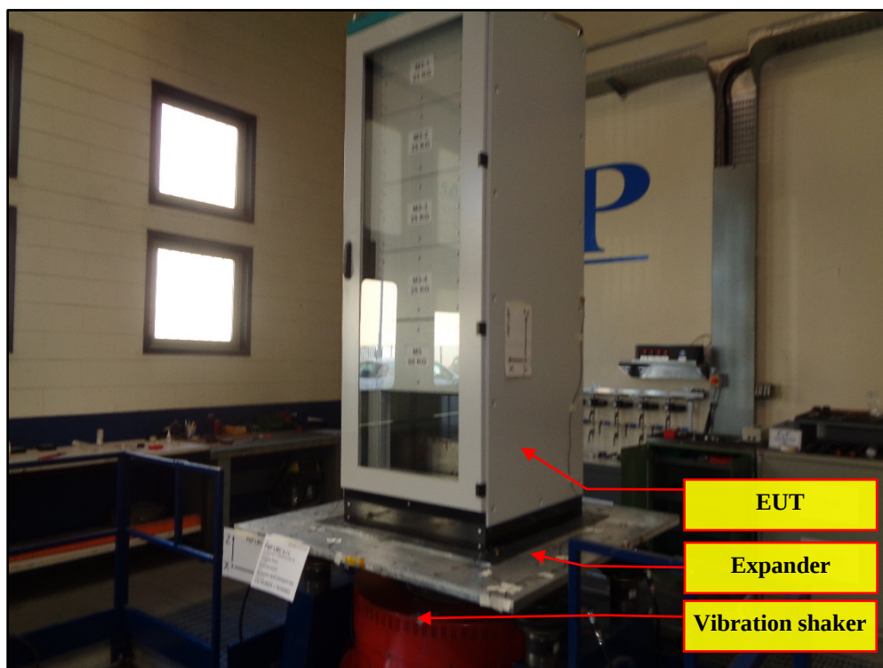
Photo 8 – Mounting technique – Z direction configuration
