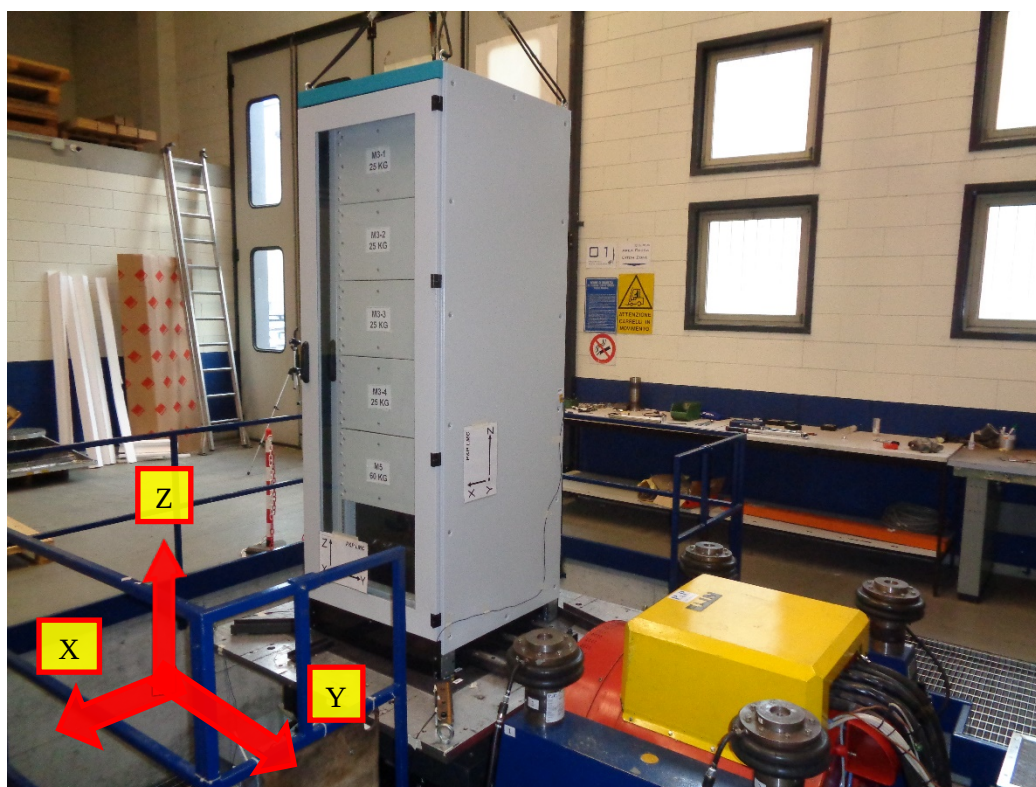
Figure 2 – Reference axis X, Y, Z of the tests
