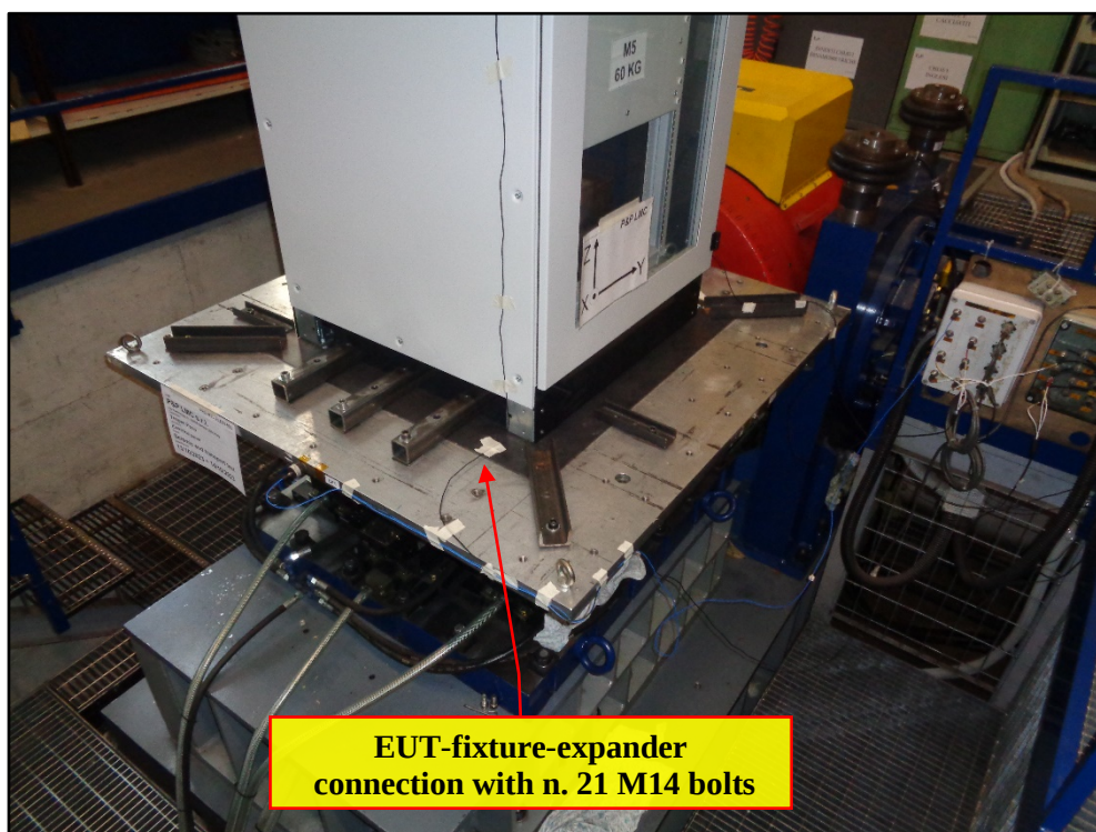
Photo 10 – Mounting technique – Fixing points of expander-Fixture-EUT
