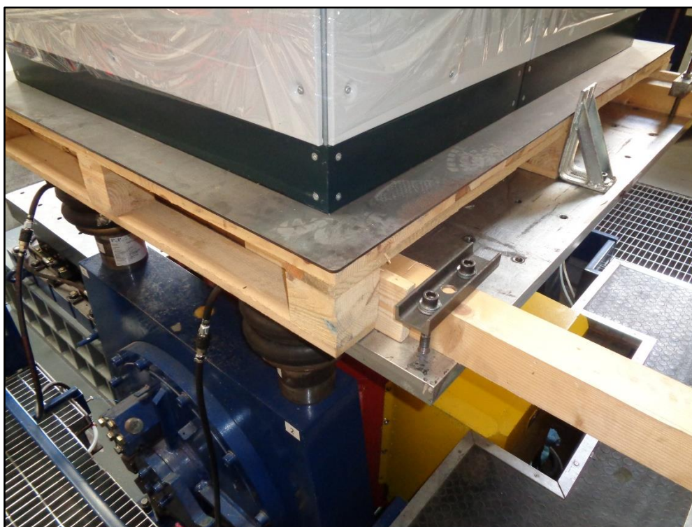
Photo 2 - Test configuration in Z direction – Constraining setup
