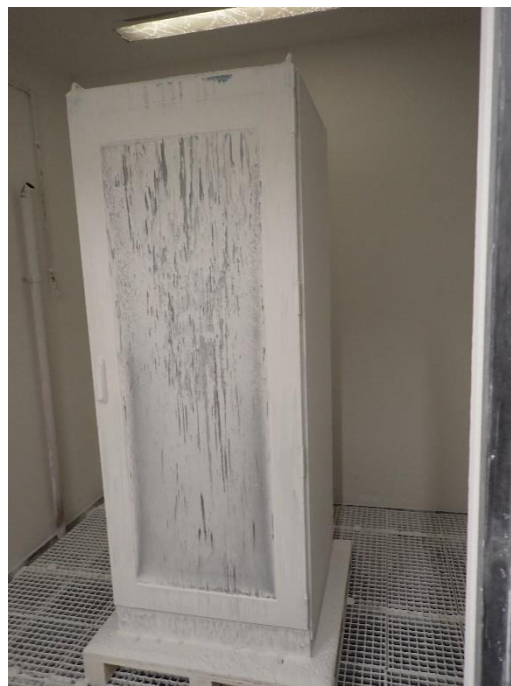
Photo 20: After IP5X test (2)
