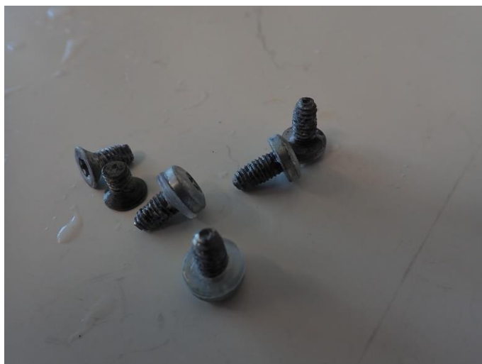
Photo 41: Samples after corrosion test (10)
