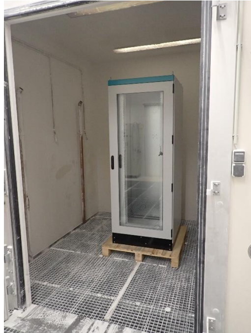
Photo 17: Before IP5X test (1)
