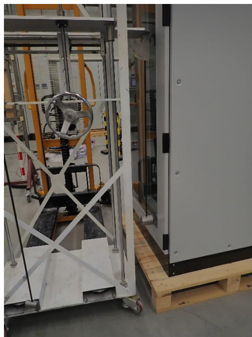
Photo 11: Mechanical impact (IK08) test (2)
