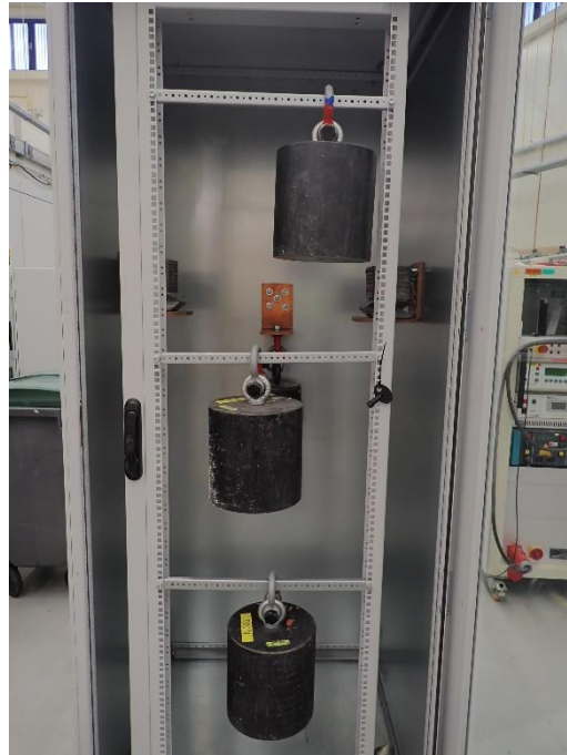
Photo 3: Static loads test (1)
