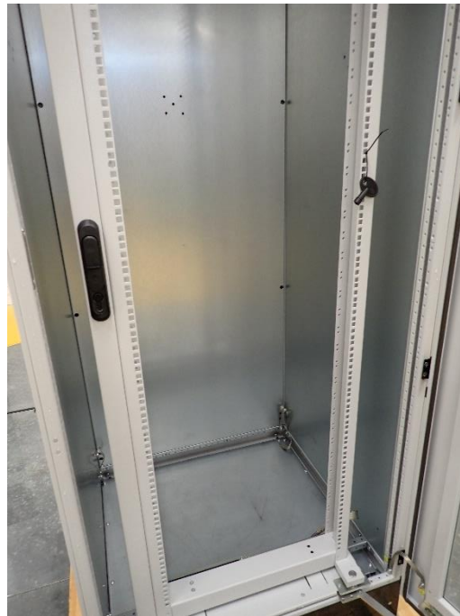
Photo 26: After IP55 test (1)
