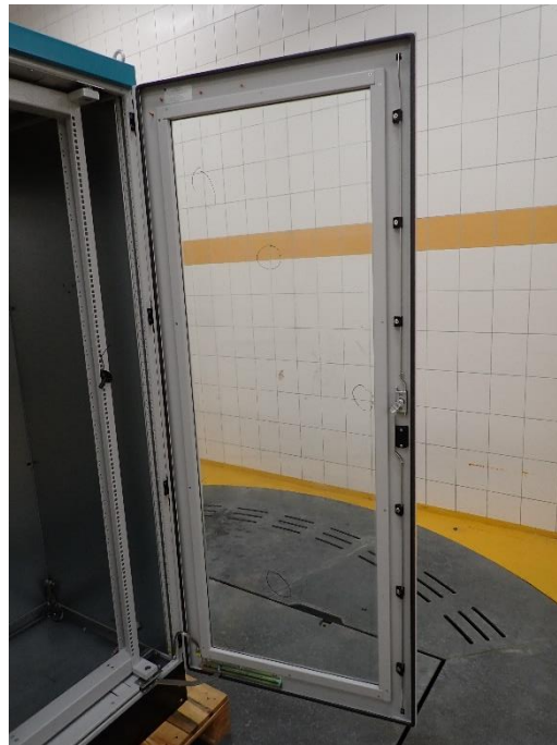
Photo 28: After IP55 test (3)
