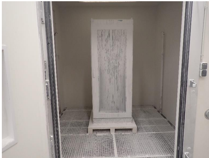
Photo 19: After IP5X test (1)
