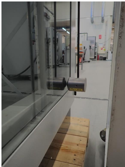
Photo 12: Mechanical impact (IK08) test (3)
