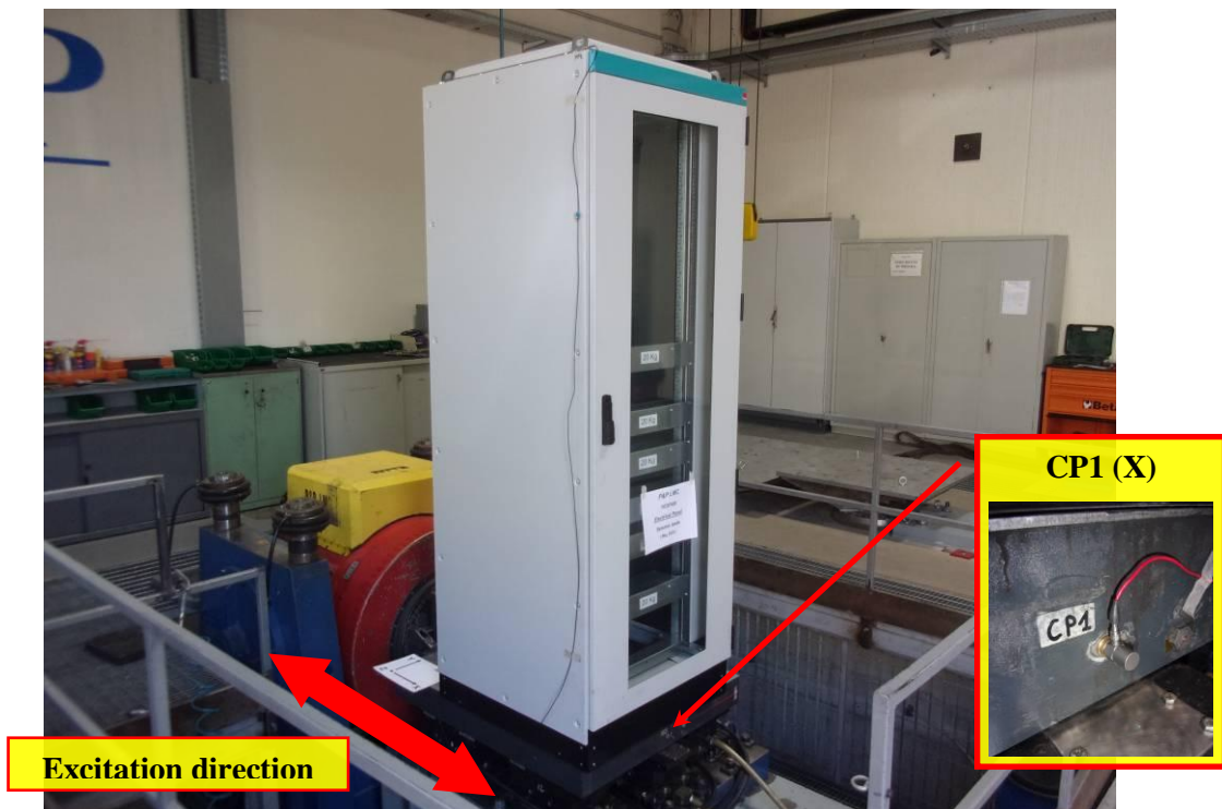
Photo 2: Test configuration for seismic test in X direction
