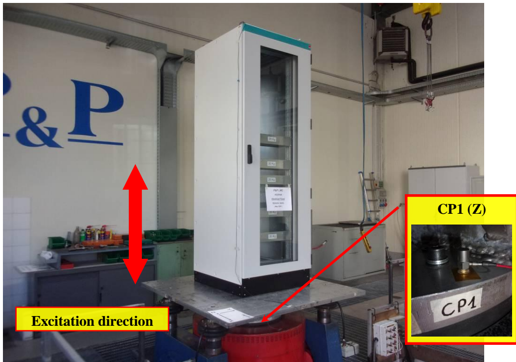
Photo 4: Test configuration for seismic test in Z direction
